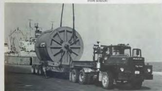
97 tonnes of rope is loaded on to "Big Habib" the special low - bed trailer.
