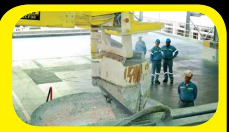
The new unit installed at Tilting Station is designed to remove maximum of solid bath and dross floating on liquid metal surface. It has majorly improved safety as with the previous unit as the work was done manually by carrying skimming tools and very close to liquid hot metal
