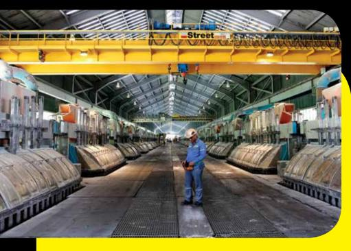
The two new overhead cranes installed in Reduction Line 1 are equipped with new arrangement of two auxiliary hoists, weighing scales and are operated by remote control. Two more new cranes will be installed to help operators work more safely and effectively.
