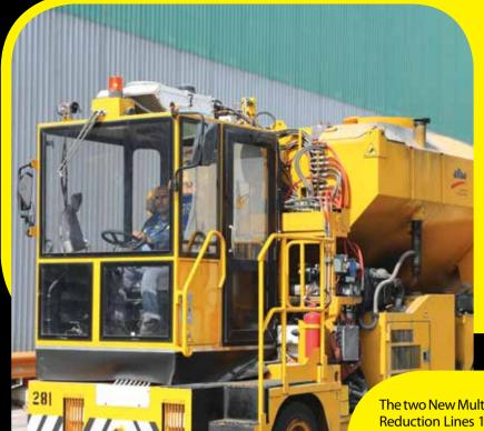
The two new fluoride charging vehicles at Lines 4 & 5 have helped to reduce the load on the multi-purpose cranes (PTA's) and improve their availability, as well as eliminated delays in fluoride charging tasks. Moreover, 12 fluoride hoppers have also been cleared from Lines 4 & 5 central passage, improving the safety conditions in this busy area.
